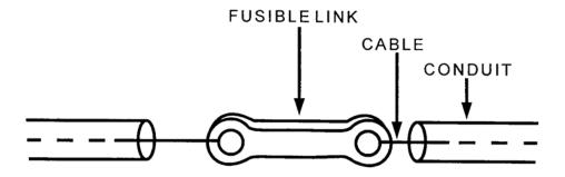
Hood range systems use a wet or a dry extinguishing agent. A dry system uses a fixed supply of dry chemical agent connected to fixed piping. Nozzles are arranged to discharge the extinguishing agent onto a burning surface. A gas, usually either carbon dioxide or nitrogen, discharges the agent under high pressure (about 350 pounds per square inch (psi)). This agent, when mixed with grease, forms a soap-like solution which helps prevent reignition.
