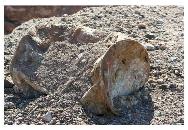
Photo No. 5—Corroded drums with deposited material containing sodium hydroxide. (SFM photo by Off. Azevedo, October 21, 2015)
