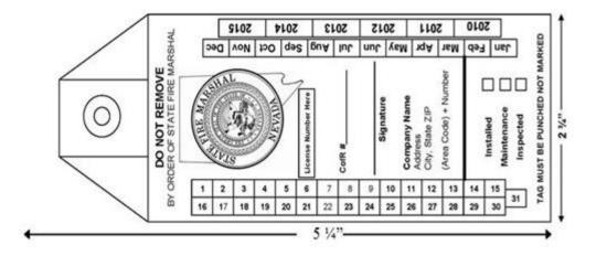
2. The tag must be attached to the system by the last person to work on the system for any purpose. The tag must be punched in an approved manner to indicate the type of service performed on the system and the date. The tag must be signed with a legible signature by the holder of a certificate of registration who directly supervises the work, and such information must remain permanently on the tag. A number stamp or date stamp must not be used on the tag.
