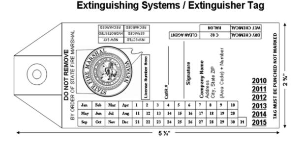
2. The tag must be punched to indicate the type of service which was performed on the *extinguisher or* system and the date on which the service was performed. Each tag must be signed with a legible signature by the holder of a certificate of registration and must be:
