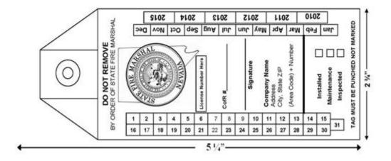
2. If the system has an outside screw and yolk valve which is not electrically supervised, the tag must serve as a seal for the valve. If the outside screw and yolk valve is electrically supervised, the tag must be attached in such a manner that the valve may be closed for testing of the supervision without removing the tag.
