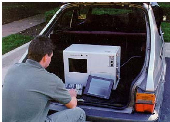
Some mass spectrometers and gas chromatographs are designed for field use .
